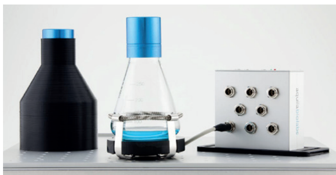
Figure 3: CGQuant and CGQ as biomass sensor component in the integrated system for biomass monitoring in shake flask cultures from INFORS HT.
