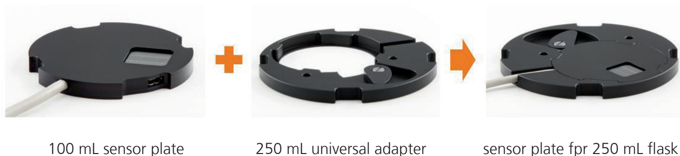
Figure 2: One CGQ sensor plate monitors each kind of shake flasks using a suitable universal adapter.
