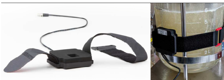
Figure 7: CGQ BioR with mounting belt - unmounted (left) and mounted (right).
