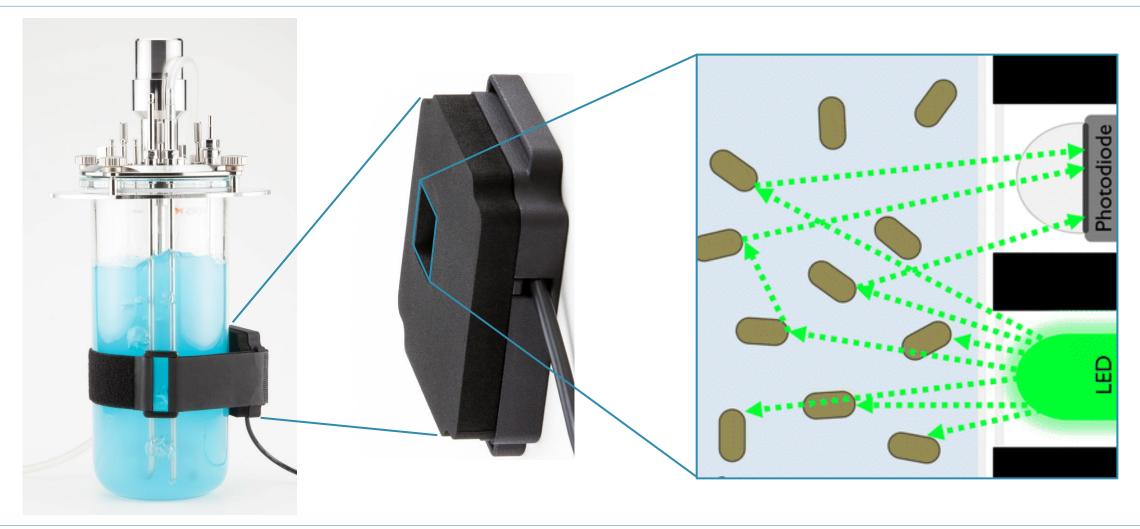
The CGQ BioR is mounted to the outside of the reactor vessel and is compatible with the majority of bioreactors (single wall and double wall).
