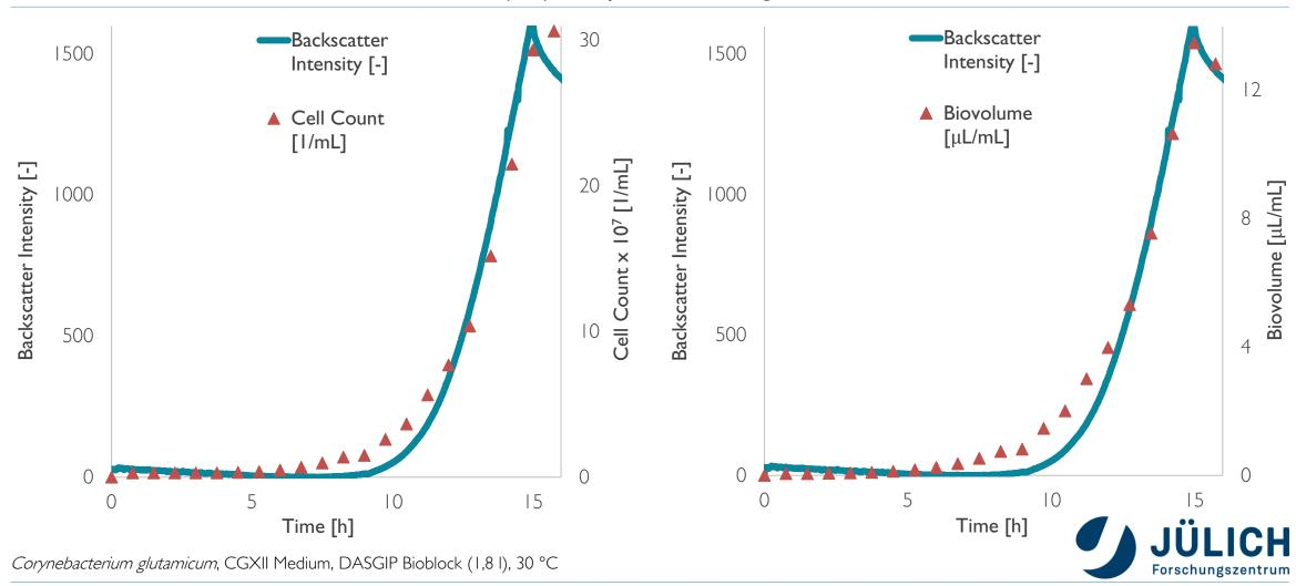
Using a calibration file, the CGQ BioR is able to directly convert backscatter measurements to OD values.
