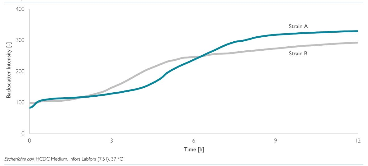
The CGQ BioR allows for non-invasive online biomass monitoring in glass bioreactors with a double wall.
