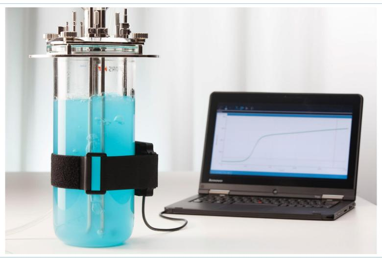
Backscatter measurements are used to monitor the biomass non-invasively through the wall of the bioreactor.
