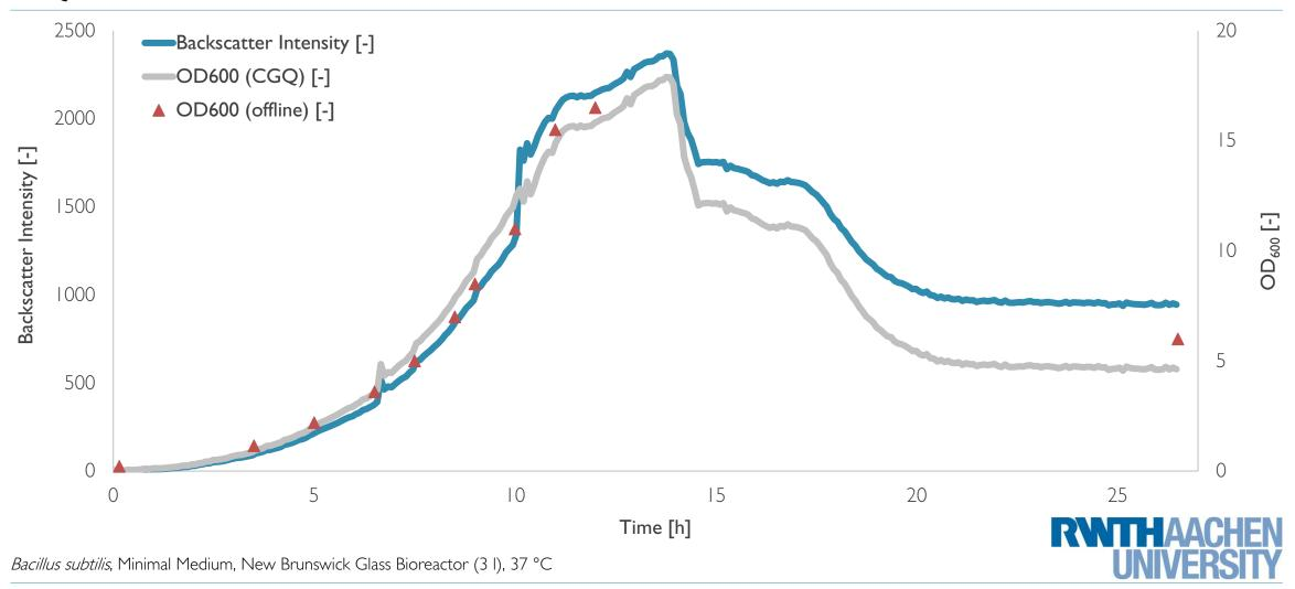
The CGQ BioR is ideal for screening experiments in bioreactors such as strain or media comparisons.
