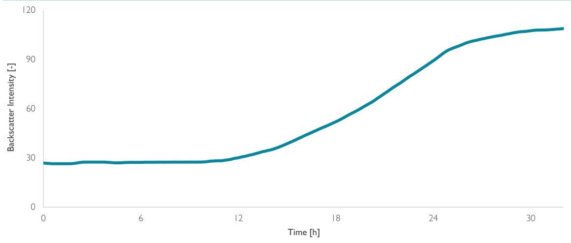
Escherichia coli BL21, M9 Medium, Applikon Glass Bioreactor (7,51), Room Temperature
